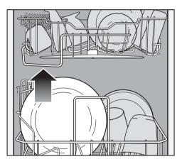
The guide at the front of the upper basket determines the maximum height for items placed in the lower basket so that the middle spray arm is not blocked. Various removable inserts are available for the lower basket to accomodate special items to be washed.
